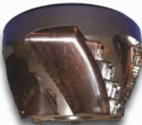
Combination Milling Cutter that Creates a Profile
